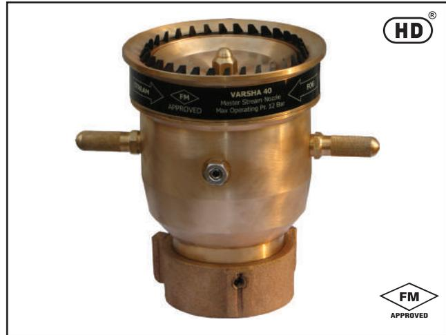
Clean the nozzle and reassemble. While re-assembling the nozzle or as a normal preventive maintenance, water proof lubricant must be used on seal and moving parts for smooth operation. The nozzle must be operated periodically under full flow straight stream and for fog pattern.
