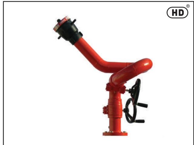
Both vertical and horizontal movements are controlled with hand wheel driven worm gears fully enclosed and protected from the elements.
